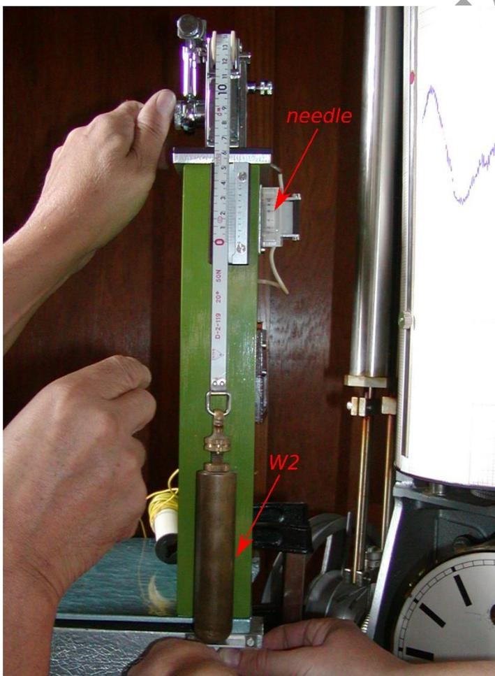
**Figure 3.** An instrument used to measure distance from the contact point level to the water surface. The smaller weight  $W1$  (not shown) is placed in the water and connected to an electrical circuit with the instrument. The moment the bigger weight ( $W2$ ) touches the water, the electrical circuit closes which is signaled by a sound and needle movement. In the figure, check is made whether the tip of the weight  $W2$  is at the level of the contact point when zero is read on the meter.
