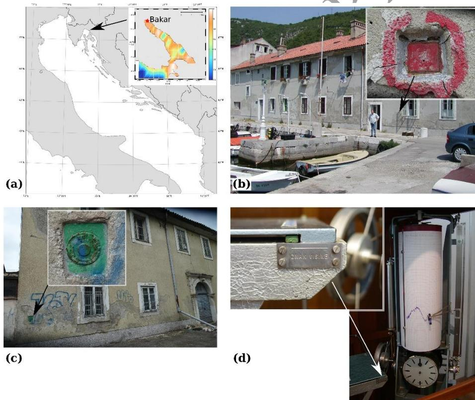
**Figure 1.** (a) The Adriatic Sea. Smaller inset shows bathymetry of the Bakar Bay and exact location of the tide-gauge station (red star). (b) Front side of the Bakar station and bench mark BV15663. (c) Back side of the station and bench mark A510. (d) Mechanical instrument and contact point.
