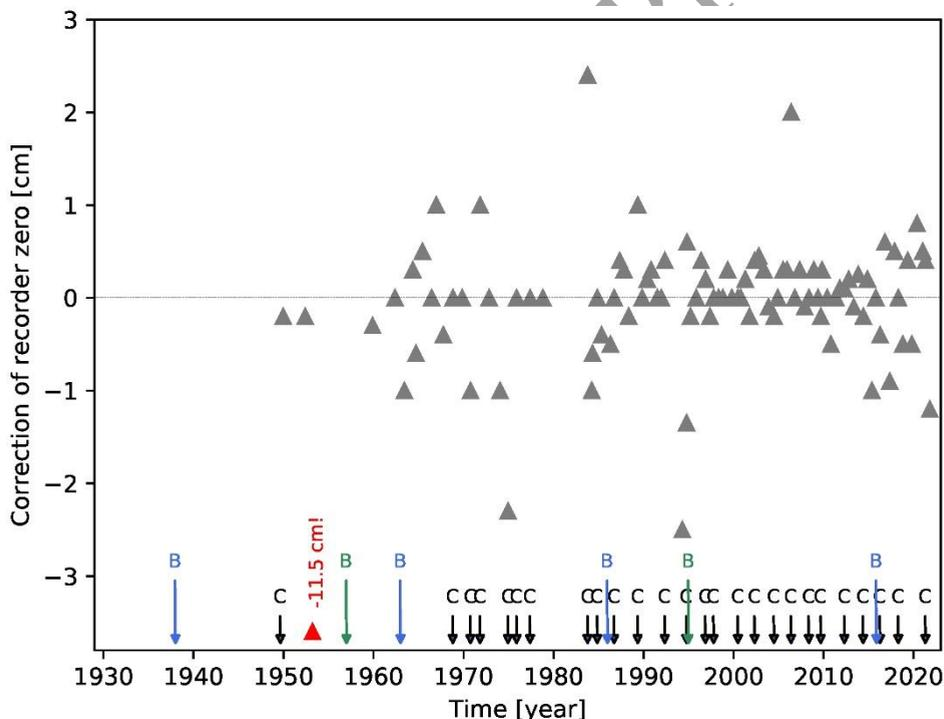
**Figure 5.** History of station maintenance over the 1929–2021 interval. Gray triangles indicate recorder-zero corrections. Red triangle marks correction of -11.5 cm, moved upward to fit the figure. Black arrows indicate cleaning of stilling well and of connecting pipe. Blue arrows indicate levelings of bench marks BV15663 and A510 (Fig. 2); green arrows indicate levelings of bench mark BV15663 and MCXVI.
