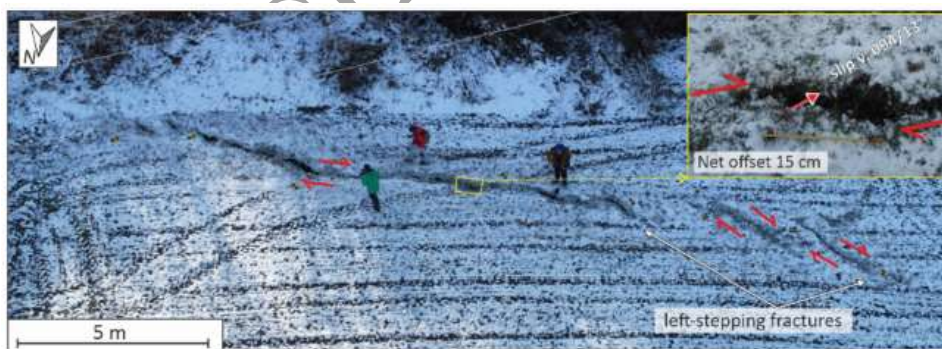
Figure 17. Aerial view (drone survey) of a ~20-m-long surface rupture on alluvial fan gravels mapped southwest of Križ Hrastovački (from Baize et al., 2022). Surface faulting occurred as a continuous rupture, striking 120°, or as a set of left-stepping en échelon ruptures. The maximum coseismic offset, measured between well-preserved piercing points, is ~15 cm.
