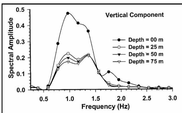
**Figure 10.** Fourier spectra of vertical component of ground displacement recorded at receiver R15 (7.5 km north of epicentre) corresponding to arrival of Rayleigh wave for different depths of submersed island.
