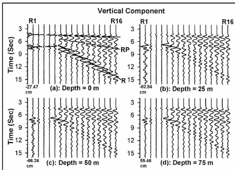
**Figure 9.** Vertical component of ground displacement for submersed island at different depths. The notations P, S, RP and R in plot 'a' (left side) illustrate P-wave, S-wave, reflected P-wave from ocean bottom and Rayleigh wave, respectively. The notations used to show the identified seismic phases are also applicable for other plots of this figure.
