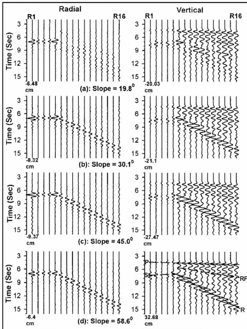
**Figure 7.** Radial and vertical components of ground displacement for different island slopes. The notations P, S, RP and R in plot 'd' (right side) illustrate P-wave, S-wave, reflected P-wave from ocean bottom and Rayleigh wave, respectively. The notations used to show the identified seismic phases are also applicable for other plots of this figure (Note: Normalization factor for vertical component is ten times larger than that of radial component)
