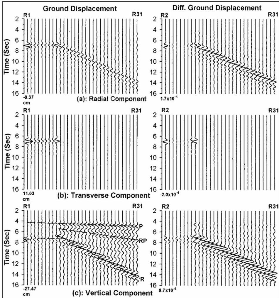
**Figure 2.** Radial, transverse and vertical components of ground displacement and differential ground displacement. The notations P, S, RP and R in plot c (left side) illustrate P-wave, S-wave, reflected P-wave from ocean bottom and Rayleigh wave, respectively. The notations used to show the identified seismic phases is also applicable for other plots of this figure (Note: Normalization factor for vertical component is ten times larger than that of horizontal component).
