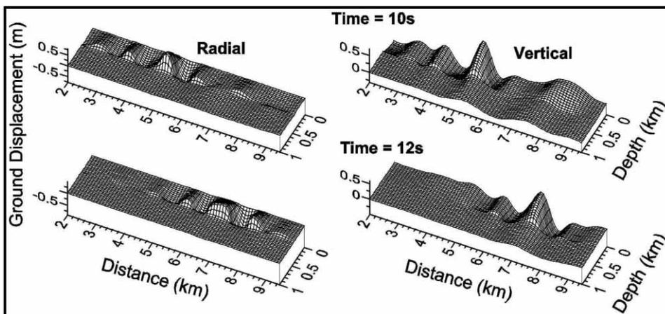
**Figure 4.** Snapshots of radial and vertical components of ground displacement in a vertical rectangular plane ( $7.5 \text{ km} \times 1.0 \text{ km}$ ) at 2.0 km north of island centre.
