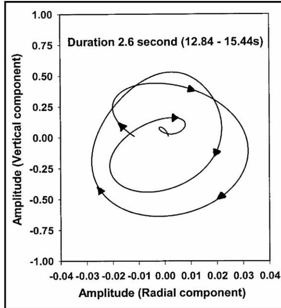
**Figure 3.** The path of particle motion at the water surface during the propagation of Rayleigh wave in a time window (12.84 – 15.44 s) and at an epicentral distance of 7.5 km towards north. The ground displacement in the radial and vertical components at different moments is plotted on X- and Y- axis, respectively.
