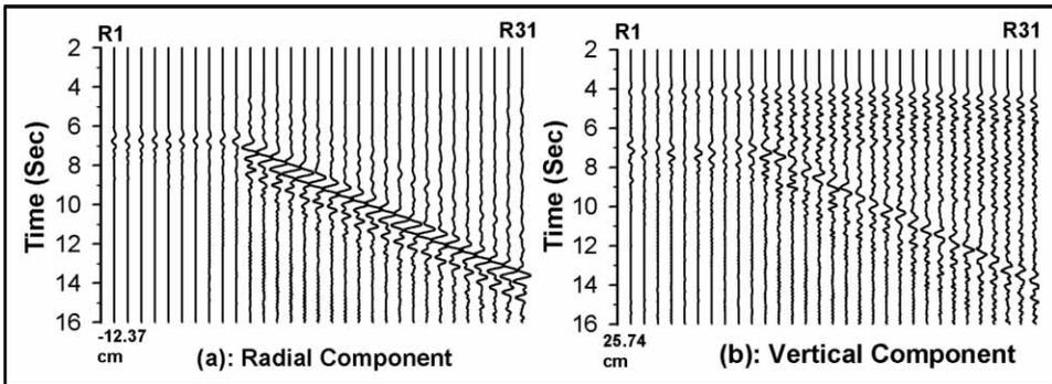
Figure 6. Radial and vertical components of ground displacement recorded at a depth of 400 m with the same source and receiver configuration as in figure 2. (Note: the criteria followed to show/identify the different seismic phases are also same as in figure 2.
