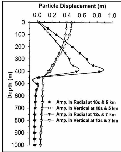
Figure 5. Rayleigh wave amplitude variation with depth at two locations.
