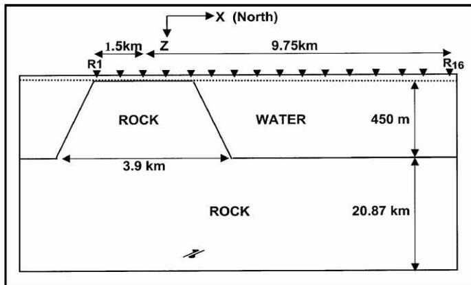
**Figure 1.** Vertically exaggerated island model (Note: two close parallel arrows show the double-couple point source).
