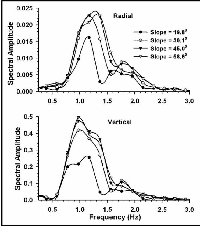
**Figure 8.** Fourier spectra of recorded ground displacement at receiver R15 (7.5 km north of epicentre) in radial and vertical components corresponding to Rayleigh wave arrival for different island-slope.
