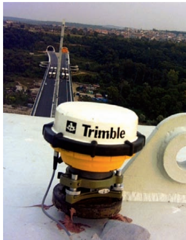
Figure 6. Displacement was measured using GPS technology.
