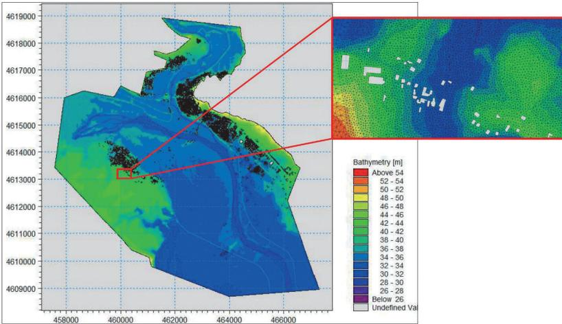
**Figure 6.** Mesh file and more sensitively generated flexible mesh at urban areas.
