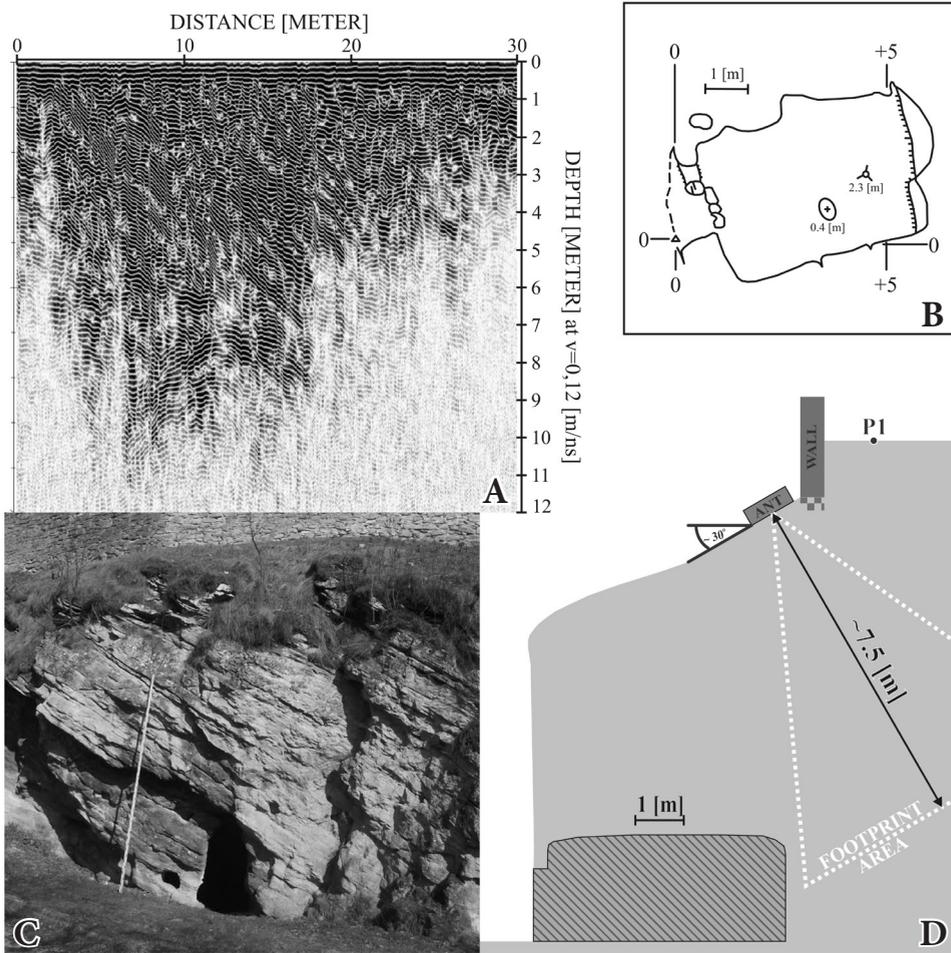
**Figure 4.** *A* – Radargram fragment from the profile number 15 imaging stratification and cave’s ceiling. *B* – Plan of the Szydło’s Cave I (Gubala et al., 1998). *C* – Opening entrance of the Szydło’s Cave I with a visible stratification of limestone (a 4 m geodesic patch makes it easier to assess the size scale). *D* – Scheme showing the methodology of measuring on escarpment and the way electromagnetic waves spread.
