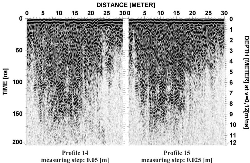
**Figure 2.** Radargrams fragments from profiles 14 and 15 documenting differences between GPR recording, depending on the type of the measuring step.
