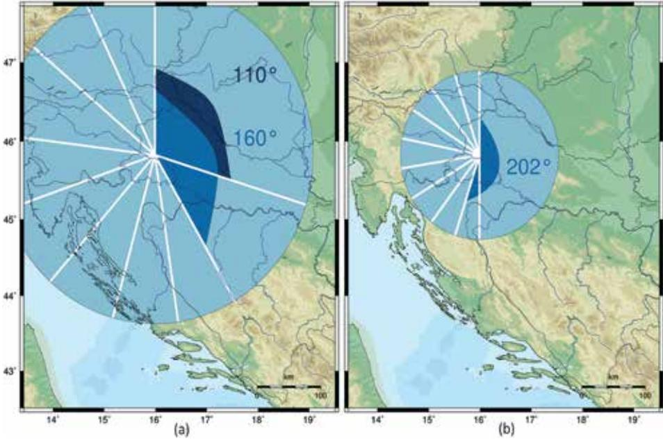
**Figure 7.** An example of a seismic network which meets the criteria: (a) from 2004; (b) determined by this paper. The white lines represent the possible station locations and the light blue area is the area within which all network stations must be. The crossover  $P_g / P_n$  distance is: (a) 250 km, which is too large for the studied area; (b) 125 km. The darker blue colours mark the limits on the primary and secondary azimuthal gaps.
