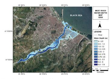
Figure 12. Water depth thematic map for a Mert River Q500 discharge.
