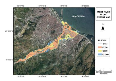
Figure 10. Flooding extent map for the Mert River for Q100, Q500, and Q1000 scenarios.
