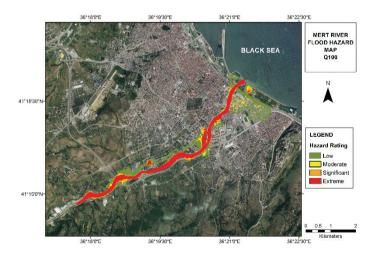
Figure 14. Flood hazard thematic map for the Mert River for a Q100 discharge.
