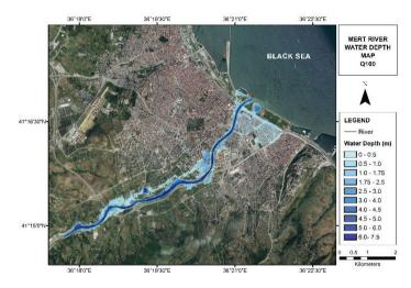
Figure 11. Water depth thematic map for a Mert River Q100 discharge.
