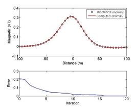
**Figure 2.** Synthetic magnetic anomaly over the sphere model (black circles in the upper graph) and generated magnetic from the MTLBO inversion (red curve in the upper graph). The lower graph illustrates the error improvement versus iteration number for the sphere model.
