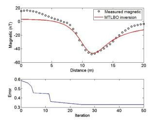
**Figure 9.** Observed total magnetic anomaly (black circles in the upper graphs), MTLBO inverted magnetic anomaly (red curve in the upper graphs) and error improvements versus iteration number (lower graphs) due to Mesozoic diabase dyke, Parnaiba basin, Brazil.
