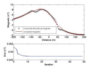
**Figure 7.** Total synthetic magnetic anomaly over a deep-seated thin sheet structure (anomaly 1) as main causative source and two neighboring sphere models (anomalies 2 and 3) as interference causative masses (black circles in the upper graph). The red curve in the upper graph shows the generated magnetic from the MTLBO inversion. The lower graph illustrates the error improvement versus iteration number for the composite model.
