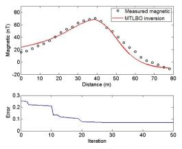
**Figure 12**. Observed vertical magnetic anomaly (black circles in the upper graphs), MTLBO inverted magnetic anomaly (red curve in the upper graphs) and error improvements versus iteration number (lower graphs) due to the Magnetite deposit from the Kerman area, Iran.
