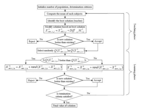
Figure 1. Flowchart of MTLBO algorithm.
