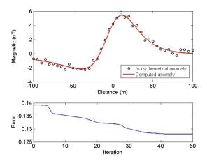
**Figure 5.** Noisy corrupted synthetic magnetic anomaly over the horizontal cylinder model (black circles in the upper graph) and generated magnetic field from the MTLBO inversion (red curve in the upper graph). The lower graph illustrates the error improvement versus iteration number for noise corrupted data of the horizontal cylinder model.
