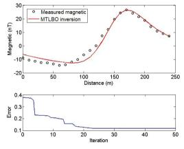
**Figure 11**. Observed vertical magnetic anomaly (black circles in the upper graphs), MTLBO inverted magnetic anomaly (red curve in the upper graphs) and error improvements versus iteration number (lower graphs) due to the Magnetite deposit from the Tabas area, Iran.
