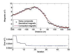
**Figure 8.** Noisy total synthetic magnetic anomaly over a deep-seated thin sheet structure (anomaly 1) as main causative source and two neighboring sphere models (anomalies 2 and 3) as interference causative masses (black circles in the upper graph). The red curve in the upper graph shows the generated magnetic from the MTLBO inversion. The lower graph illustrates the error improvement versus iteration number for noise corrupted data of the composite model.
