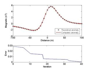
**Figure 4.** Synthetic magnetic anomaly over the horizontal cylinder model (black circles in the upper graph) and generated magnetic from the MTLBO inversion (red curve in the upper graph). The lower graph illustrates the error improvement versus iteration number for the horizontal cylinder model.
