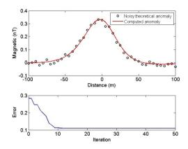
**Figure 3.** Noisy corrupted synthetic magnetic anomaly over the sphere model (black circles in the upper graph) and generated magnetic from the MTLBO inversion (red curve in the upper graph). The lower graph illustrates the error improvement versus iteration number for 10% noise corrupted data of the sphere model.
