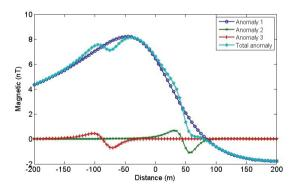
**Figure 6.** Total magnetic anomaly generated by a deep-seated thin sheet structure (anomaly 1) as main causative source and two neighboring sphere models (anomalies 2 and 3) as interference causative masses.
