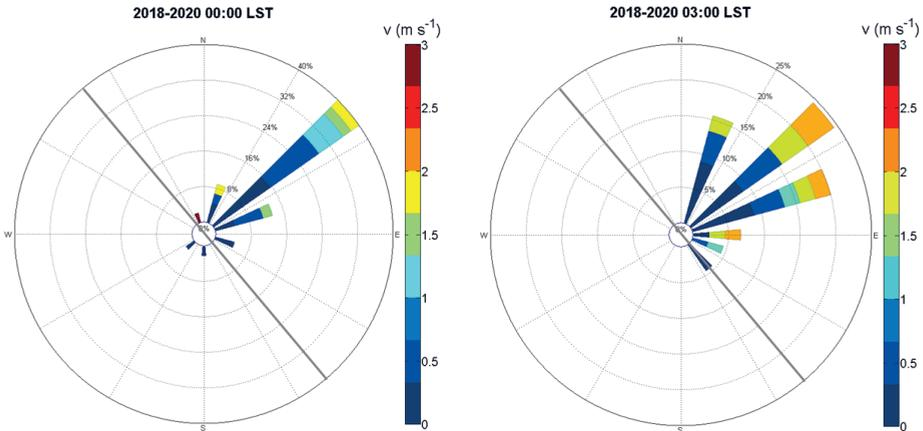
**Figure 4.** Diurnal variation of wind rose for days with an LLB. Corresponding times are given in local standard time (LST, without summertime advancement by 1 h). Grey solid line shows direction of the main lake axis.
