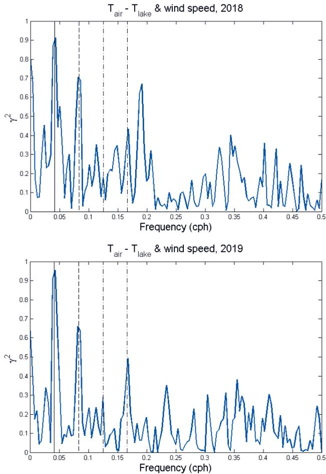
**Figure 9.** The magnitude-squared coherence ( $\gamma^2$ ) between the hourly mean wind speed and the hourly mean land-water temperature difference. The vertical solid, dashed, dashed-dotted, and dotted lines correspond to periods of 24, 12, 8, and 6 h, respectively. Values for 2020 could not be determined since some of the air temperature data for this year were missing.
