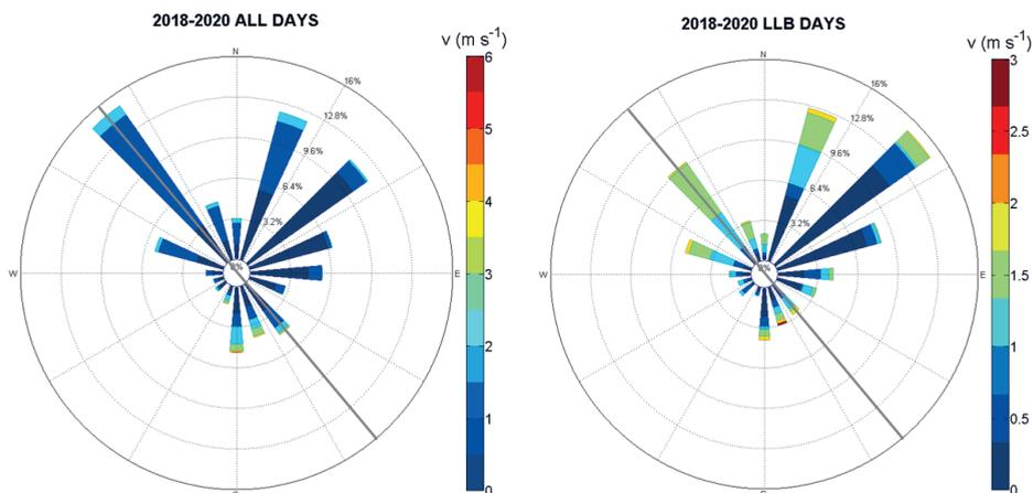
**Figure 3.** Wind roses for all analyzed days (*left*) and for days with an LLB (*right*). Grey solid line shows direction of the main lake axis. Note that the range of wind speed values for all days is twice as large as that for LLB days.
