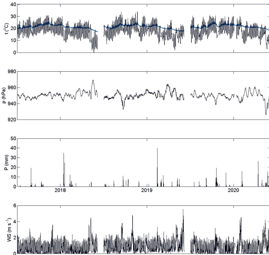
**Figure 2.** Observed hourly values of the air and lake temperature at a depth of 0.2 m ( $t$ , black and blue lines, respectively), air pressure ( $p$ ), precipitation amount ( $P$ ), and wind speed ( $WS$ ) for 8 July–30 September of 2018–2020.
