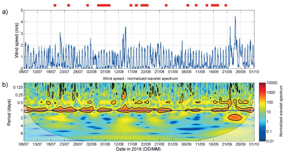
**Figure 5.** Wind speed (Panel *a*) and the corresponding normalized wavelet spectrum (Panel *b*) for summer 2018. Time intervals that satisfy LLB Conditions 1–7 listed in Section 3 are indicated in red above the Panel *a*. The horizontal blue line in Panel *b* corresponds to a period of 24 h. The thick black line indicates the 95% confidence level, with red noise as the background spectrum. Lighter shadings on both ends in Panel *b* denote regions where edge effects become important.
